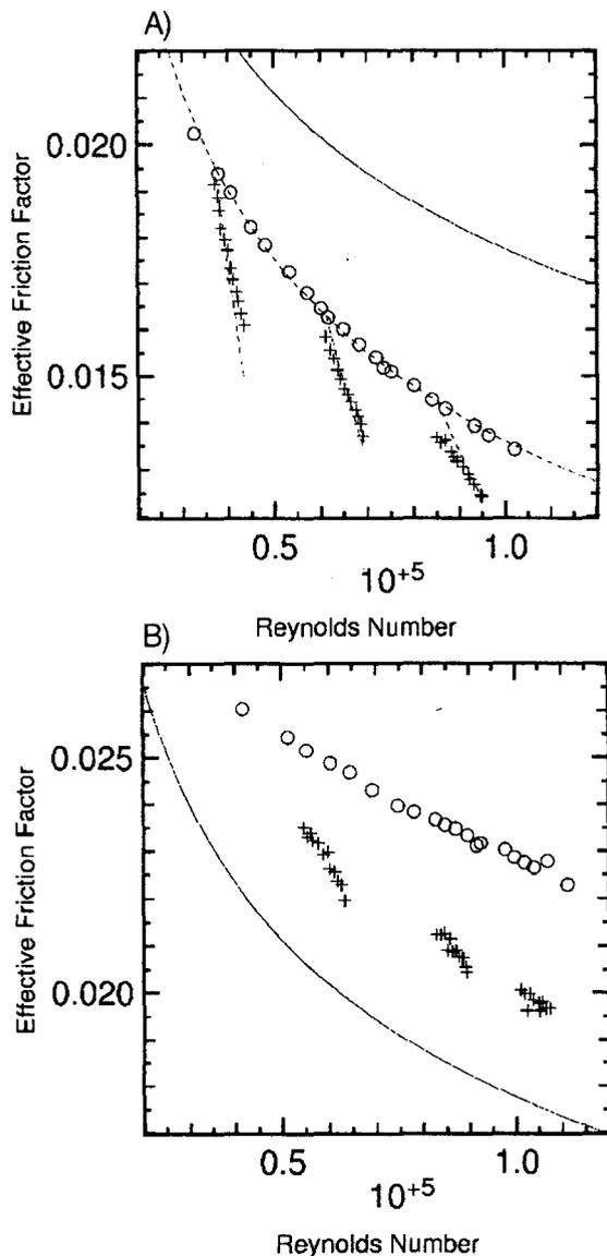
Fig. 7—Effective friction factor for T pipe downstream of the perforated section: (A) Section 4, just downstream of the perforated section, (B) Section 3.
