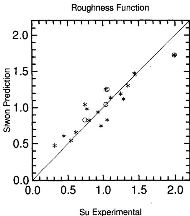
Fig. 4—The roughness function determined from the Siwoń model (Siwoń 1987) (asterisks) plotted with respect to the roughness function determined by Su (1996). The circles are described in the text.
