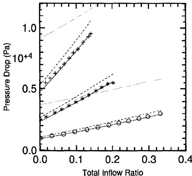
Fig. 6—T test data, Siwoń model predictions (solid lines), and modified Yuan et al. model predictions (dotted and dashed lines).
