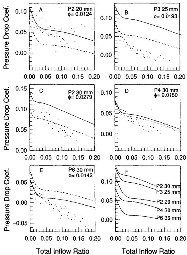
Fig. 10—Comparison of the pressure-drop coefficient using the Chen friction factor (solid) and the pipe-specific Su friction factor (dashed).
