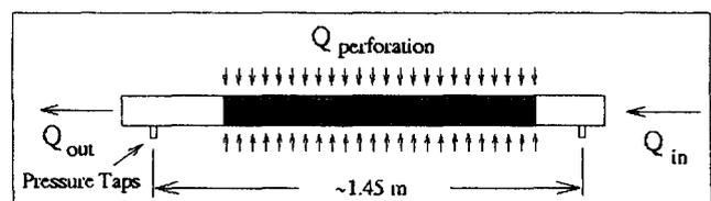
Fig. 8—Test configuration for the P pipe series of experiments [after Su (1996)].
