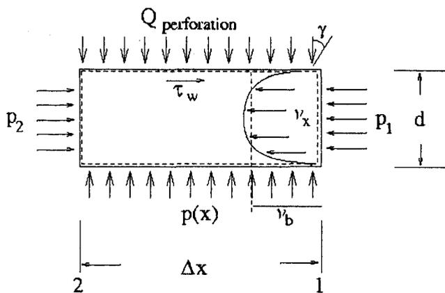
Fig. 1—Control volume for a section of perforated pipe.
