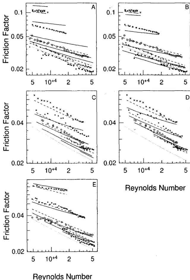
Fig. 11—Experimental data of Yuan (1997) and model fits of Yuan et al. (1999) (solid lines) and Siwoń (1987) (dashed). The dotted line represents a smooth pipe.
