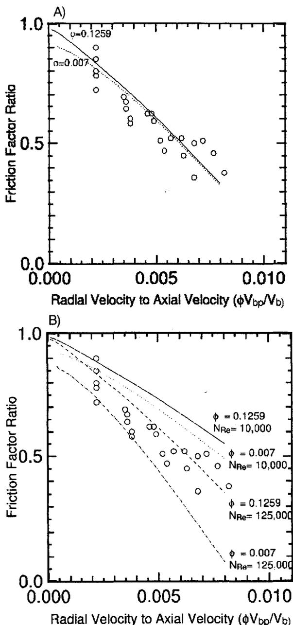
Fig. 2—Plots of Siwoń model and Olson and Eckert data: (A) with the no-inflow friction factor determined by Olson and Eckert; (B) with friction factors determined using Siwoń's correlation.
