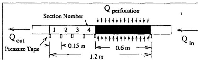
Fig. 5—Experimental setup for T tests [after Su (1996)].
