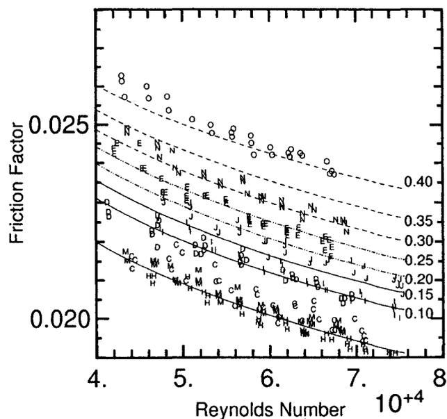
Fig. 3—Comparison of model predictions (lines) to experimental results (letters).
