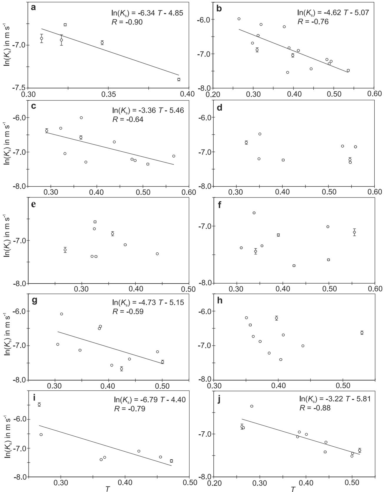
**Figure 5.** (a–j) Observed correlation between collocated measurements of hydraulic conductivity  $\ln(K_s)$  and WSP texture  $T$  for subsections 1 through 10 of the Fanshawe section. Linear regression is presented only for those subsections for which the correlation coefficient exceeds the critical value at the 95% significance level. Vertical bars indicate the measurement error associated with hydraulic conductivity.
