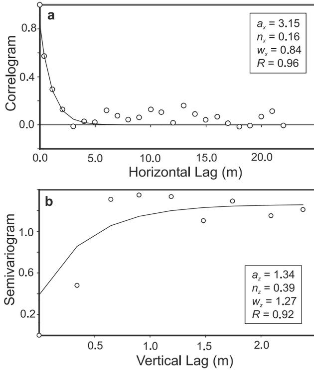
**Figure 7.** Experimental and model geostatistics for log-transformed hydraulic conductivity. (a) Horizontal correlogram. (b) Vertical semivariogram. Points indicate calculated geostatistical values based on core permeameter measurements; solid lines indicate the optimum least squares solutions corresponding to the listed model parameters.
