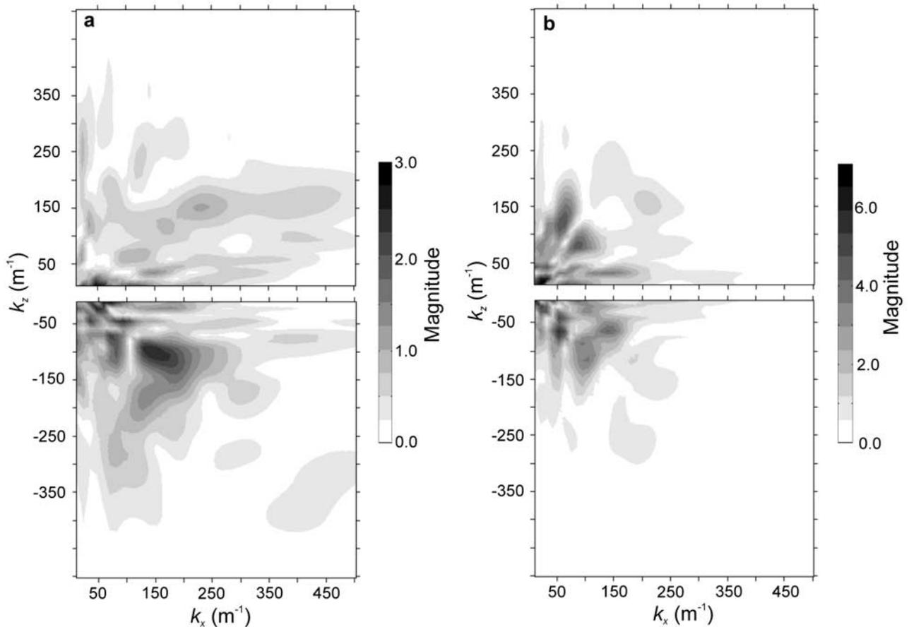
**Figure 2.** Local S spectrum magnitude  $S_{xz}(k_x, k_z)$ . (a) Fine-grained S spectrum at the coordinates  $x = 8.45$  m,  $z = 2.35$  m. (b) Coarse-grained S spectrum at the coordinates  $x = 6.95$  m,  $z = 1.00$  m.
