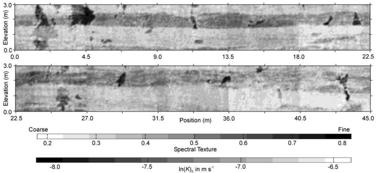
**Figure 3.** Spectral texture map and estimated log-transformed hydraulic conductivity field for the Fanshawe section.
