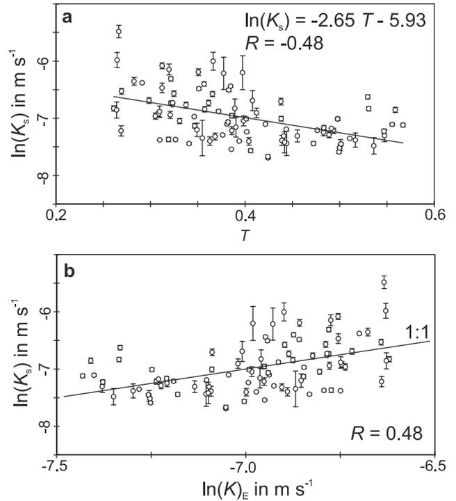
**Figure 6.** (a) Observed correlation between collocated measurements of hydraulic conductivity  $\ln(K_s)$  and WSP texture  $T$ . (b) Measured versus estimated hydraulic conductivity. Vertical bars indicate the measurement error associated with hydraulic conductivity.
