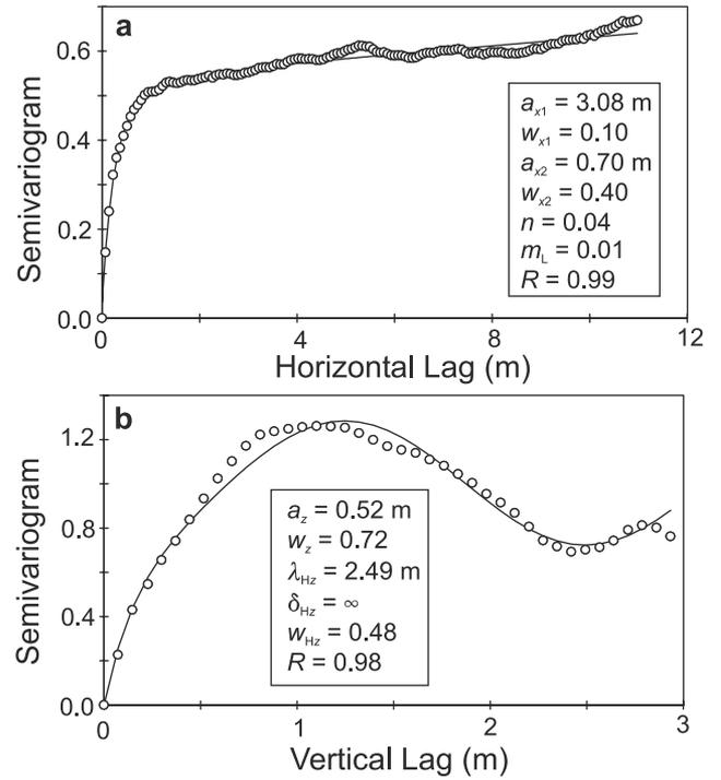
**Figure 8.** Experimental and model geostatistics for the spectral texture map of the Fanshawe section. (a) Horizontal semivariogram. (b) Vertical semivariogram. Points indicate calculated geostatistical values based on WSP texture; solid lines indicate the optimum least squares solutions corresponding to the listed model parameters.
