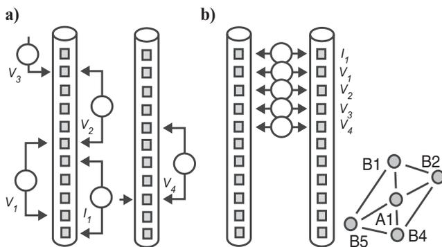
Figure 4. Schematic representation of survey geometries.  $I_1$  indicates the first current dipole and  $V_i$  indicates the  $i$ th potential dipole for that current dipole. (a) Circulating skip-3 vertical dipole-dipole: multiple passes are made with the potential dipole through all boreholes in order to address every possible electrode pair with the given skip separation. (b) Horizontal dipole-dipole: data are collected in an arrangement of two-borehole panels as shown to the right.
