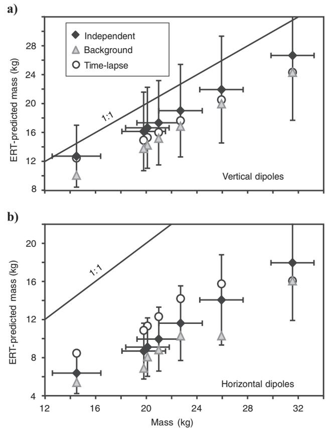
Figure 12. Comparison of total solute mass in the aquifer obtained from water sample measurements with that predicted by ERT for the three inversion protocols. (a) Vertical and (b) horizontal dipole data (note the different scale). Error bars are illustrated for the independent inversion protocol only.
