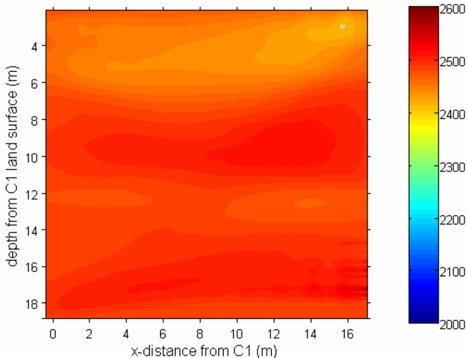
**Figure 6:** Tomogram generated using crosswell data collected at the BHRS.
