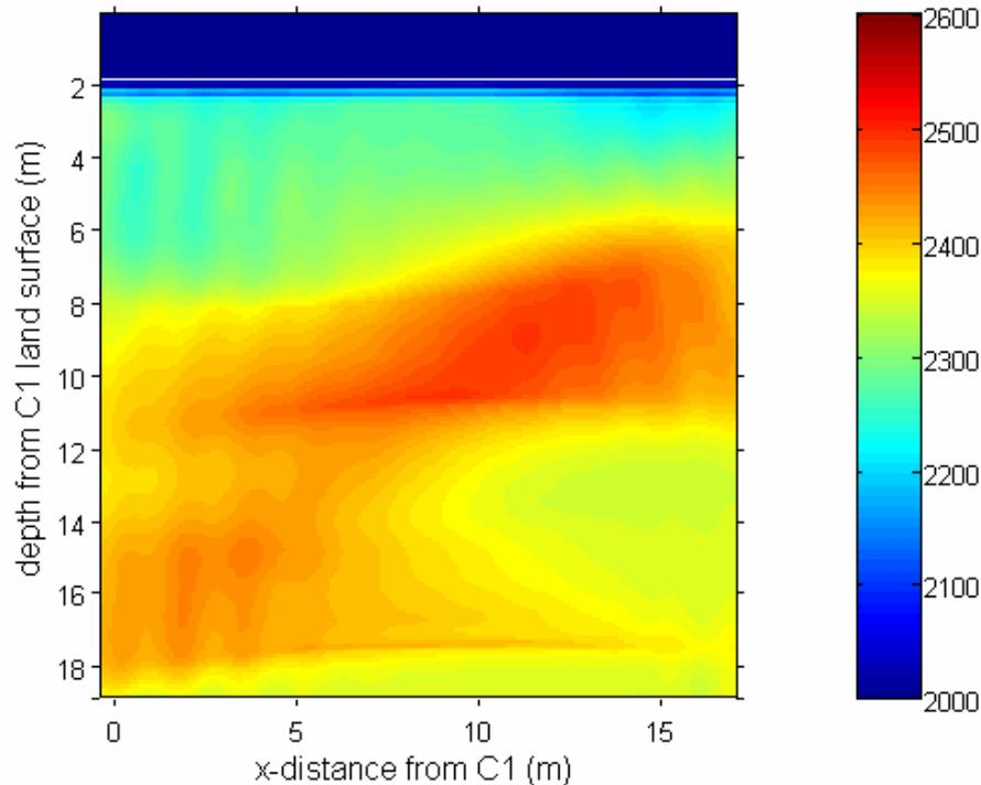
**Figure 7:** Tomogram generated using crosswell and borehole-to-surface data collected at the BHRs. The velocity above 1.95 m is within 5 m/s of 330 m/s.
