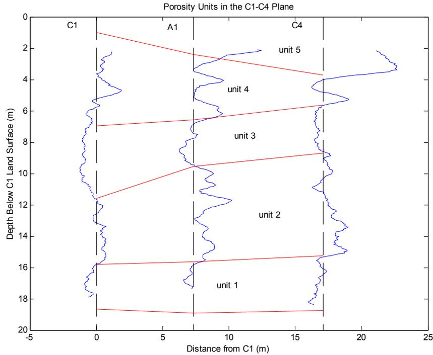
**Figure 5:** Interpreted porosity units in the C1-C4 plane. The vertical dashed lines are the well locations, and also represent 0.20 on the porosity logs. The depth of the unit 4-unit 5 boundary in well C1 is arbitrary because unit 5 is not present in the C1 porosity log.
