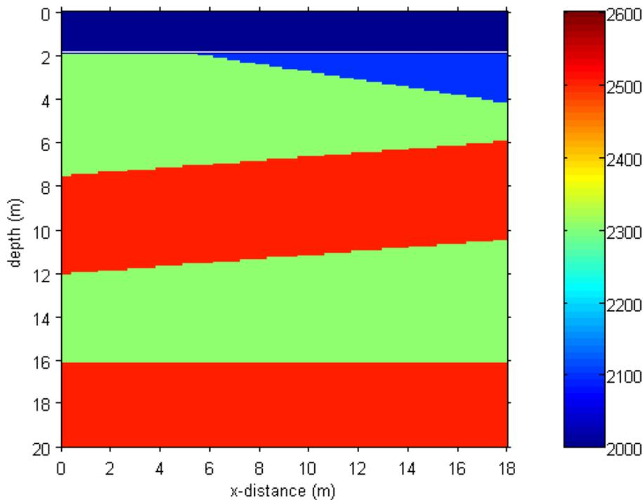
**Figure 1:** Velocity model used to generate synthetic data. The velocity is 330 m/s above 1.95 m depth.
