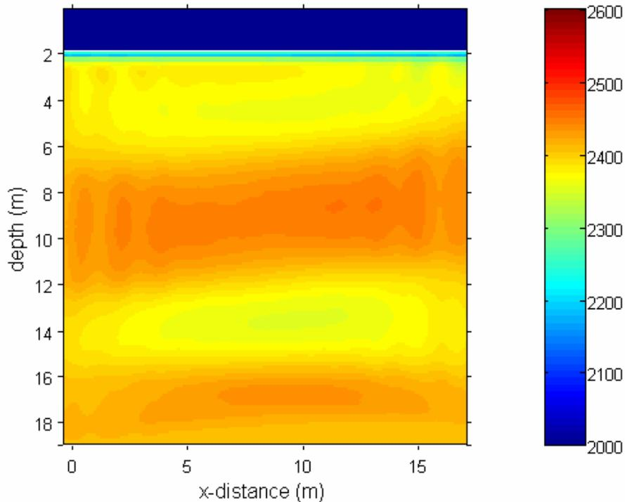
**Figure 3:** Tomogram generated using synthetic crosswell and borehole-to-surface data. The velocity above 1.95 m is within 5 m/s of 330 m/s.
