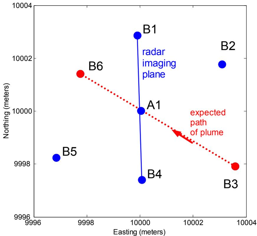
**Figure 1.** Map of the central portion of the BHRS showing the injection well (B3), the withdrawal well (B6), the twenty-zone multilevel sampling well (A1), and the surrounding monitoring wells (B1, B2, B4, B5, and B6) with log-through capability. The distance between wells B1 and B4 is 5.57 m; the distance between wells B3 and B6 is 6.90 m.
