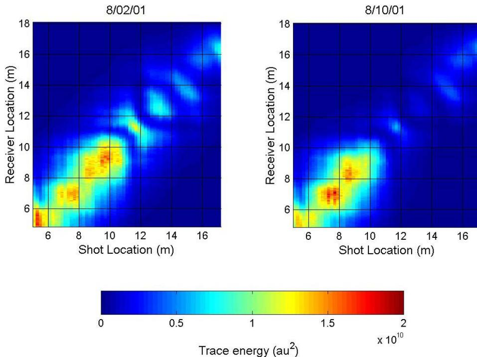
**Figure 5.** Trace energy on August 2 and August 10, 2001, plotted as a function of transmitter and receiver depths. The level run data fall along the diagonal from the lower left to the upper right. The colorbar indicates the magnitude of trace energy.
