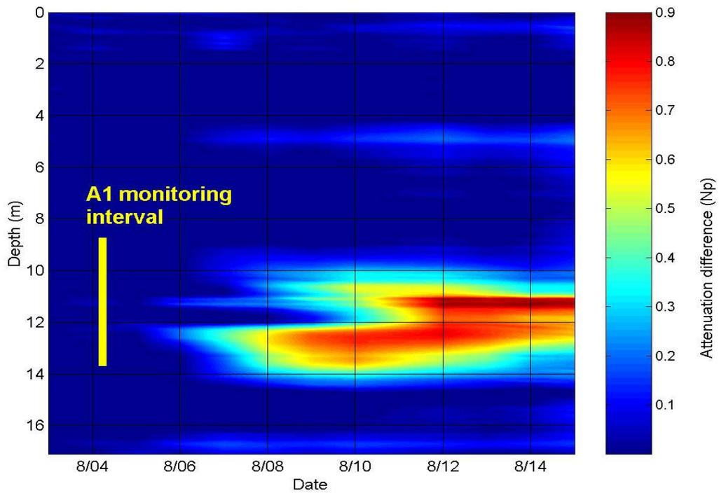
**Figure 3.** Attenuation differences for the time-lapse level run surveys (100 MHz) of the B4-B1 plane. The differences were calculated using equation (7). Data from August 2, 2001, were used as the initial conditions.
