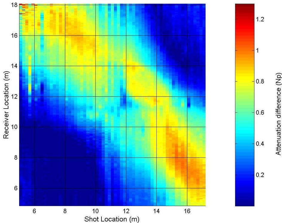
**Figure 6.** Attenuation differences between August 2 and August 10 in the B4-B1 plane plotted with respect to transmitter and receiver depths. Attenuation differences were calculated according to equation (7).
