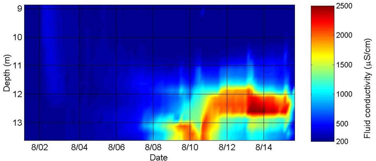
**Figure 4.** Fluid conductivity for water samples collected in well A1 (after Hausrath et al., 2002). The samples were collected from 20 zones spaced 0.25 m apart over the monitoring interval (8.75-13.75 m depth). Conductivity values have been temperature-compensated to 25 degrees C.
