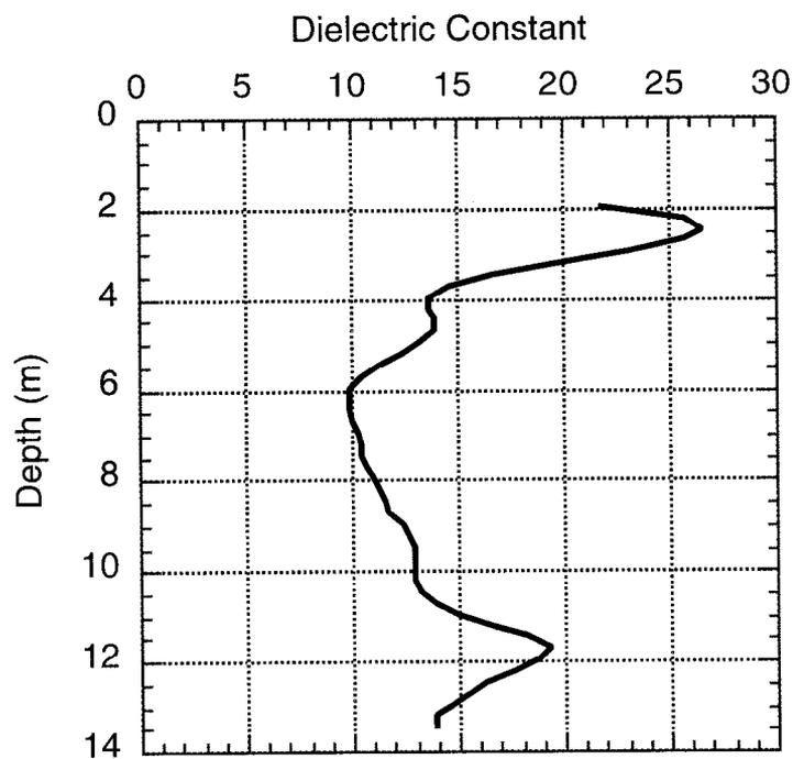
Figure 3. Dielectric constant versus depth, derived from interval velocities.
