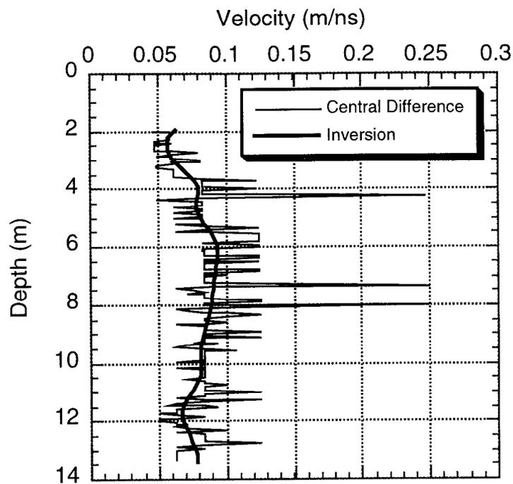
Figure 2. Interval velocity versus depth, derived from first-arrival traveltimes.
