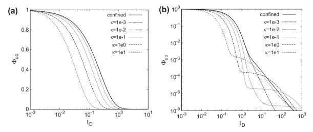
**Fig. 13.** Plots of dimensionless head,  $\Phi_{uc}(t_D)$ , computed with the kinematic boundary condition at the water table, against dimensionless time,  $t_D$ , on (a) semi-log and (b) log-log scale, for different values of the anisotropy ratio,  $\kappa$ , with  $S_v = 0.3$ , with d = 0.0 m and l = 0.3 m.
