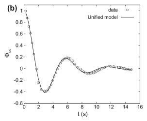
**Fig. 10.** Linear plots of model fit to BHRS B5 slug test data in test intervals (a) 8.69–8.99 m (overdamped) and (b) 10.21–10.51 m (oscillatory) below the measuring point;  $K_{r,1} = 2.0 \times 10^{-4} \text{ m s}^{-1}$ .
