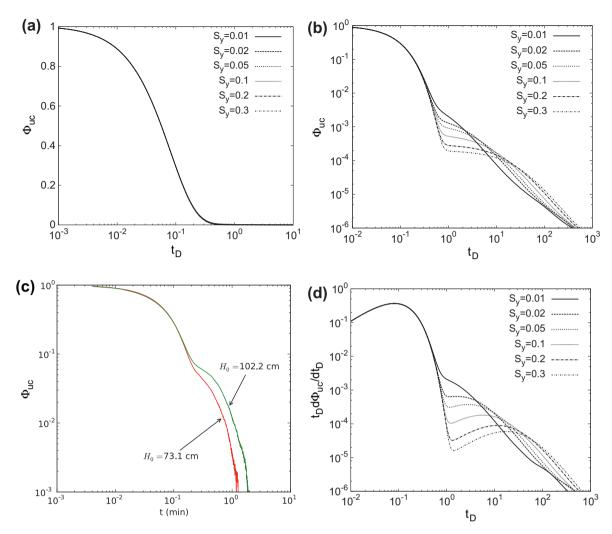
**Fig. 12.** Plots of dimensionless head,  $\Phi_{uc}(t_D)$ , computed with the kinematic boundary condition at the water table, against dimensionless time,  $t_D$ , on (a) semi-log and (b) loglog scale, for different values of specific yield,  $S_y$ , with  $\kappa = 1.0$  with d = 1.0 m and l = 1.3 m. The plot in (c) shows slug test data collected at a site near Butte, Montana, and (d) shows the log-time/derivative of the predicted response  $\partial \Phi_{uc}/\partial \ln(t_D)$ .
