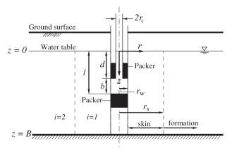
Fig. 1. Schematic of the slug-test problem flow domain.
