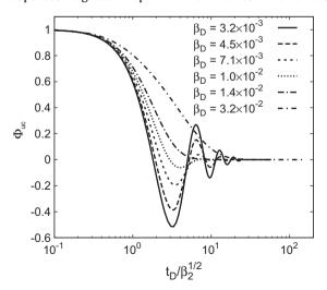
**Fig. 2.** Semi-log plot of dimensionless head,  $\Phi_{\rm uc}(t_D)$ , computed with the unified model, against dimensionless time,  $t_D/\sqrt{\beta_2}$ , for different values of the dimensionless inertia parameter  $\beta_D$ . Oscillations diminish with increasing  $\beta_D$ .
