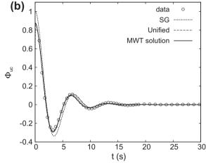
**Fig. 6.** Linear plots of model validation results. The unified and KGS solutions are fitted to field data and compared to the fits of existing models (data after McGuire (1994), Zlotnik and McGuire (1998)).
