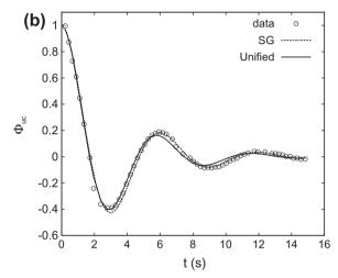
**Fig. 11.** Linear plots of model fit to BHRS B5 slug test data in test intervals (a) 8.69–8.99 m (overdamped) and (b) 10.21–10.51 m (oscillatory) below the measuring point, assuming no skin.
