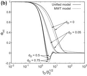
**Fig. 5.** Semi-log plots of dimensionless head,  $\Phi_{\rm uc}(t_D)$ , against dimensionless time,  $t_D/\sqrt{\beta_2}$ , for different depths  $(d_D)$  below the water table, comparing the MWT solution to (a) the confined aquifer (BZ) solution of Butler and Zhan (2004) and (b) the unified model.
