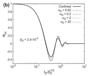
**Fig. 4.** Semi-log plots of dimensionless head,  $\Phi_{\rm uc}(t_D)$ , computed with the kinematic water table boundary condition, against dimensionless time,  $t_D/\sqrt{\beta_2}$ , for different values of the dimensionless parameter  $\alpha_D = \kappa/\sigma$ , for (a) monotonic and (b) oscillatory responses.
