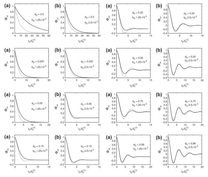
**Fig. 8.** Comparison of the unified unconfined aquifer model developed here (dotted line) with the model of Butler and Zhan (2004) (solid line) at the indicated normalized depths to test interval for (a)  $b_D = 1.25 \times 10^{-2}$  and (b)  $b_D = 2.5 \times 10^{-2}$ .
