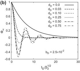
**Fig. 3.** Linear plots of dimensionless head,  $\Phi_{\rm uc}(t_D)$ , computed with the unified model, against dimensionless time,  $t_D/\sqrt{\beta_2}$ , for different values of the normalized depth below the water table,  $d_D$ , with a normalized test interval length of (a)  $b_D = 1.25 \times 10^{-2}$  and (b)  $b_D = 2.5 \times 10^{-2}$ .
