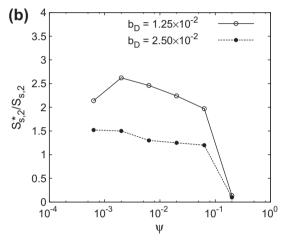
**Fig. 9.** Linear plots of (a)  $K_{r,2}^*/K_{r,2}$  and (b)  $S_{s,2}^*/S_{s,2}$  against the dimensionless parameter,  $\psi=(r_w/b)\sqrt{K_{z,2}/K_{r,2}}$ , for two different values of the dimensionless test interval length ( $b_D=1.25\times 10^{-2}$  and  $b_D=2.5\times 10^{-2}$ ), at  $d_D=0.25$ .
